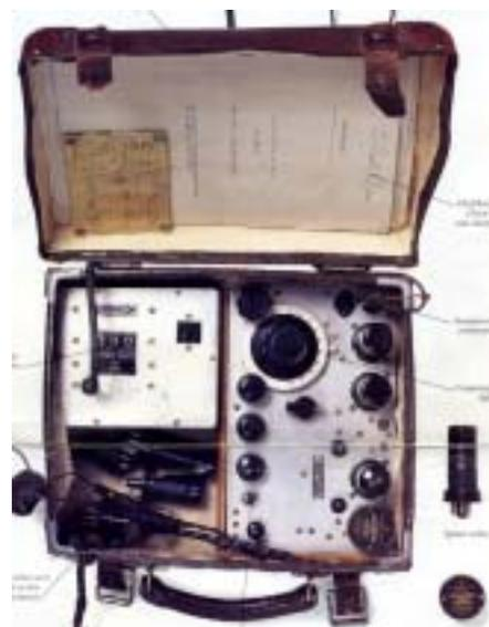
quite large variations in impedance. It seems as though there was much more thought expended on the transmitter than the receiver. It is rather crude even by 1939 standards. There is no "bandspread" tuning in this early version, nor an RF amplifier stage to isolate the detector from the antenna, nor is there any possible provision for any sort of sidetone so that it is impossible to hear your own sending.
