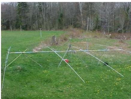
Carefully lower the two tripods, making sure that the mast is supporting the weight of the boom. Be careful that the element tips don't dig in to the ground. Depending on how high the boom plate is off the ground you may not have to completely lower the tripods, you just need to get them down enough so that you can check the balance.
