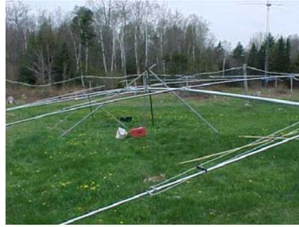
Mark the balance point at the one U bolt. Insert the second U bolt and THEN slide the boom over so the balance point is between the two bolts. At this point you can also adjust the boom to mast plate so it is perpendicular to the elements. Either use a carpenter's level or with this antenna I just used the element brace posts as a vertical reference and aligned them to the mast then tightened down the boom U bolts.
