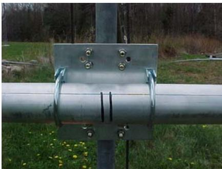
Now just raise the two assembly tripods back up to support the ends of the boom. While the temporary mast is in place the boom is level you can also set the boom brace ropes to the right lengths.
