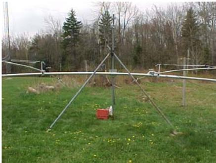
This is the whole setup with the boom still supported by the two tripods near the ends.
